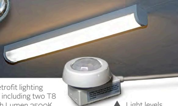
▲ Retrofit lighting fixture, including two T8 GE High Lumen 3500K lamps enclosed and gasketed with a spread beam Miro reflector, and a two-lamp F32T8 GE UltraMax 1.18 ballast factor programmed-start dimming ballast.
