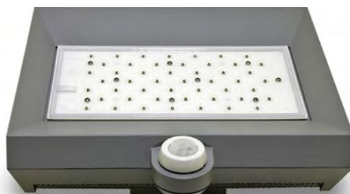
◀ 70-watt bi-level LED Emco fixtures with integrated occupancy sensors replaced 186 metal halide fixtures in the Downtown Central Garage. The LED fixtures have a rated life of 100,000 hours, over five times greater than the metal halide fixtures being replaced. City Staff consider the fixture maintenance savings an added benefit of the new LEDs.
