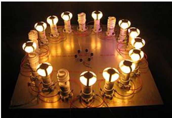
FIGURE 13. PHILIPS L PRIZE LED LAMP STRESS TESTING ALONGSIDE CFL A LAMPS
