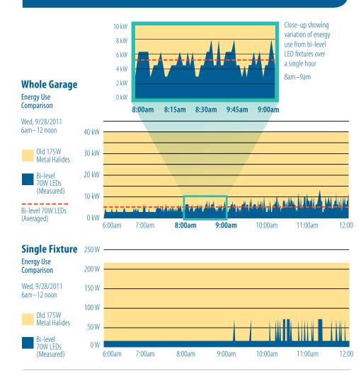
for two reasons: existing lighting is inefficient and there are often long periods of low occupancy. Retrofitting to high efficiency bi-level fixtures presents an opportunity to save energy by both reducing energy use at full light output and dimming light levels during unoccupied periods. Bi-level lighting can work in conjunction with occupancy sensors, photo sensors, wireless controls, and other scheduling or controls technologies.
